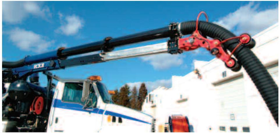
The new Vector 5x5 boom telescopes outward five feet and allows the hose to move downward an additional five feet. Movement is controlled by a convenient wireless remote (optional).
